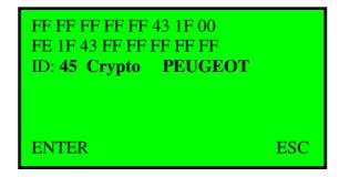
Transpronics, can copy 90% of transponders that are in Volkswagen and Ford cars, it also has detailed data about the transponder. For example, a transponder that has never programmed before has this information below. This transponder's ID part can be copied to a T5 or an ID 33 transponder but cannot start the car.
