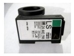
In the immobilizer unite seen above, there is a processor named TMS370C702. After this eeprom is read you have to send it to our machine. (Processor must be read as a \*Bin file)
